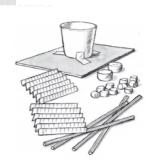
**Test, evaluate and redesign** - Drop your lander from a height of one foot (30 cm). If the "astronauts" bounce out, figure ways to improve your design. Study any problems and redesign. Once the "astronauts" stay in the aircraft consistently, add a foot to your height and try again.
